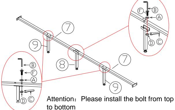
STEP 5: Loose the bolt on the headboard, then link the rail to the headboard. STEP 6:
