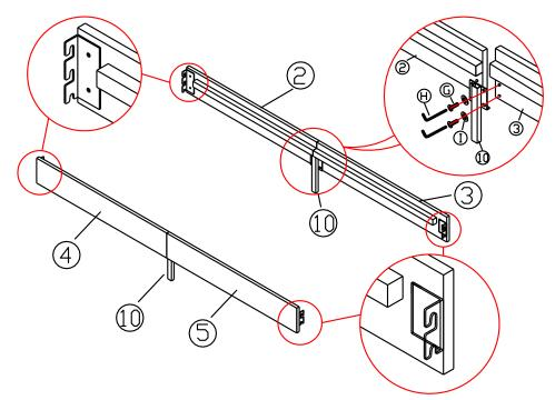
Attention: Please align the two rails tightly before tightening the bolts.
